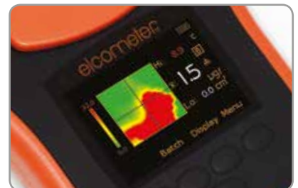
2D Salt Density Map with High/Low Readings
