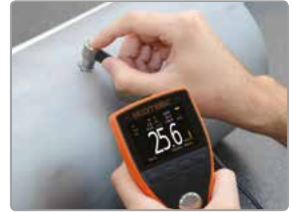
Ideal for measuring steel pipes where there is only access to one side.
