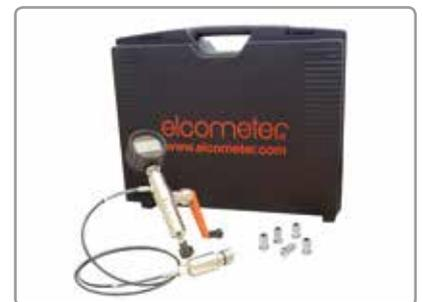
Supplied in a robust plastic carry case the kit includes the Elcometer 508 and five dollies which can be cleaned with the heated tongs and reused.
