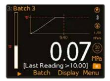
Either pull to maximum or pull to preset limit. Unique time hold feature allows users to set a delay before pressure returns to zero.
